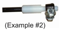
**Step 6. Attaching the aircraft cable to your towed vehicle's brake pedal.**
